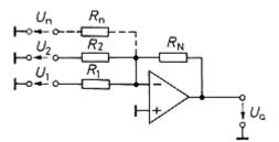
Drawing 1 - Inverting adder circuit
